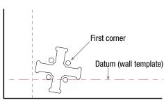
Step 5- Using the template, work your way along the wall in a horizontal orientation. Perimeter tiles should be finished on corners with ¼ clips and straight joins with ½ clips. \*Never use the tiles to measure spacing. Double check your spacing by gently offering two adjoining tiles into the clips without pushing the tiles deeply into the clips.
