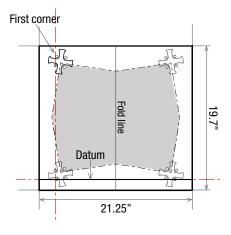
Step 2- Using hardware suitable for your substrate, fix the first corner in place.
