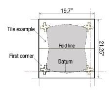
Step 4- Rotate the installation template 90° and place it over two wall clips. Ensure the rotated horizontal line of the template aligns with the wall datum. Use the template to fix the next two clips in place.
