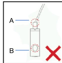
A. Direction of wire and gripper must be in a straight line
