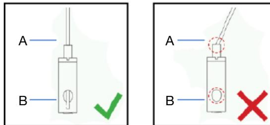
A. Direction of wire and gripper must be in a straight line
